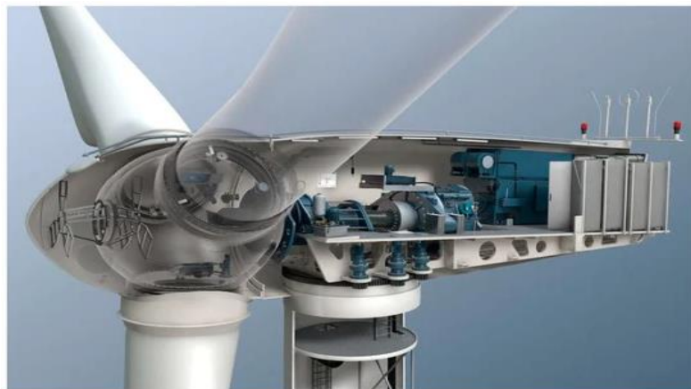
1-rasm. Shamol turbinasidagi vites qutisning ichki tuzilishi
